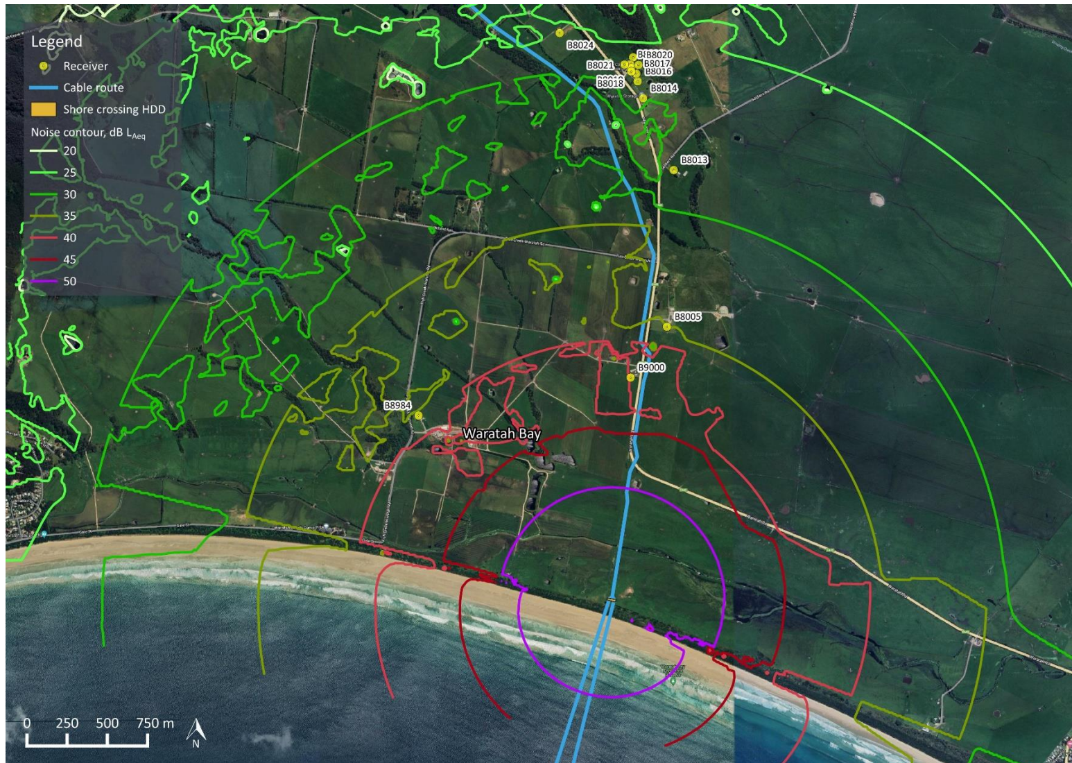
Figure 7: Shore crossing – HDD works predicted noise contours, dB L_{Aeq}
