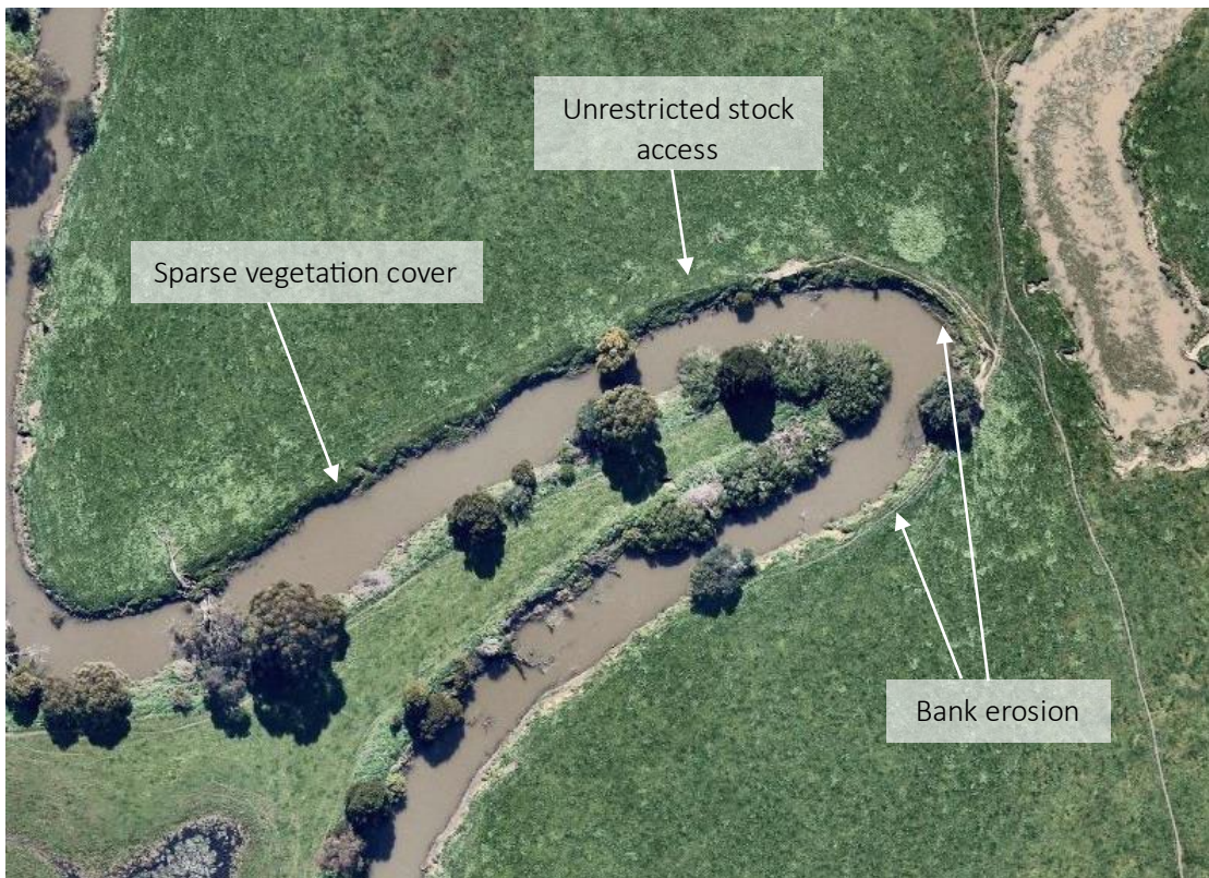
Figure 65. September 2021 aerial imagery of meander bend downstream of proposed project alignment (Nearmap).
