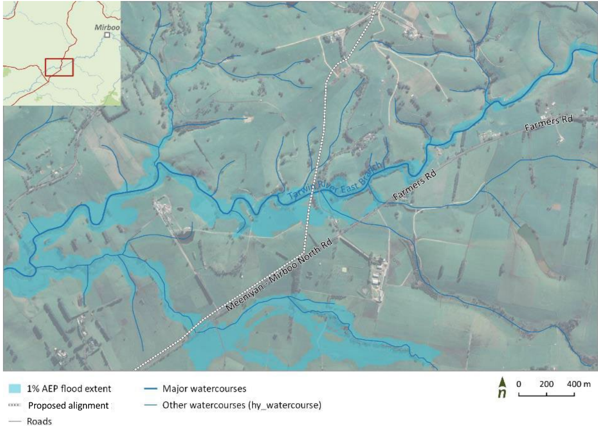
Figure 10. 1 % AEP flood extent for the Tarwin River East Branch surrounding the proposed project alignment.
