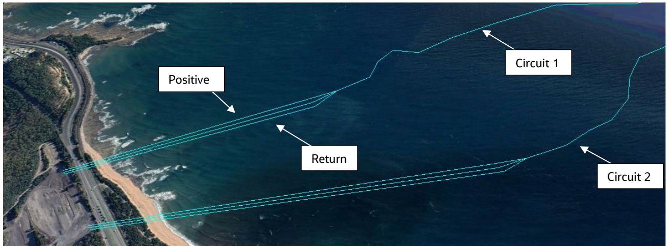
Figure 5-2: Non-uniformity of cables at the Tasmanian shoreline
